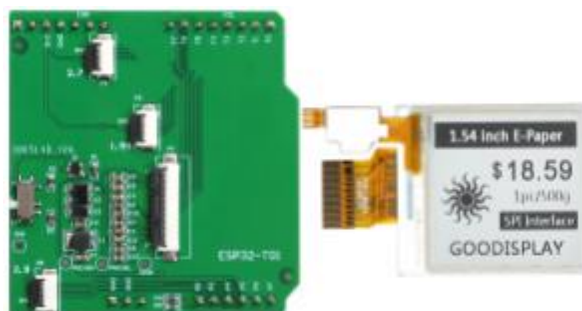
Figure 4 Connecting Adapter and E-paper display
